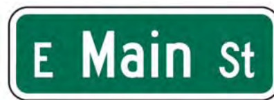
Figure 13. The street name signs in the study area (left) use the old lettering style that has now been superseded by a mixed-case style (above). Source: 2009 MUTCD.
