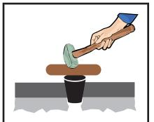
Place a PLUG-R® in the hole, cover with a board and pound in with a hammer.
